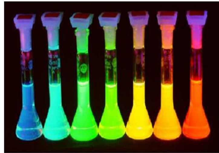
Quantum dot fluorescence (Q-dots) CdSe of various sizes when exposed to UV light
