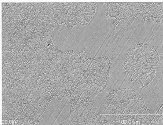
Fig. 23. Surface of \text{Ni}_3\text{Al} phase subjected to electrocorrosion process: 500x
