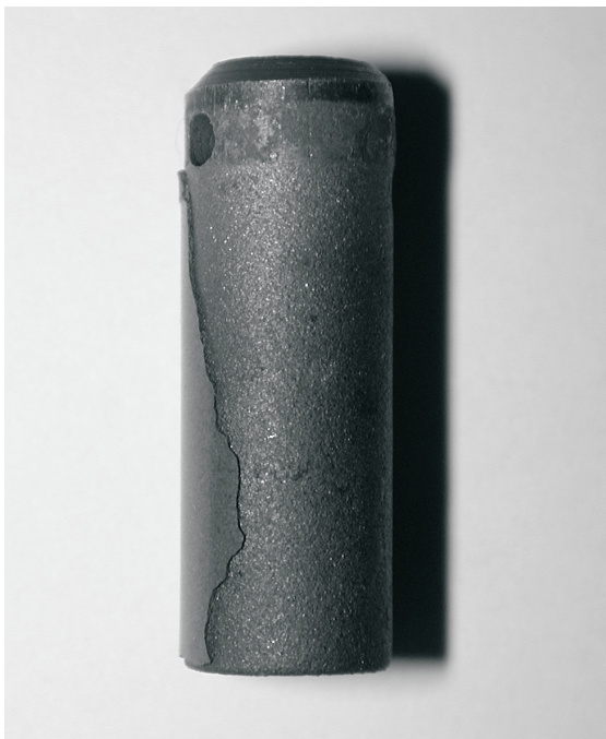
Fig. 7. Rupture of the coating Al 2 O 3 -TiO 2
