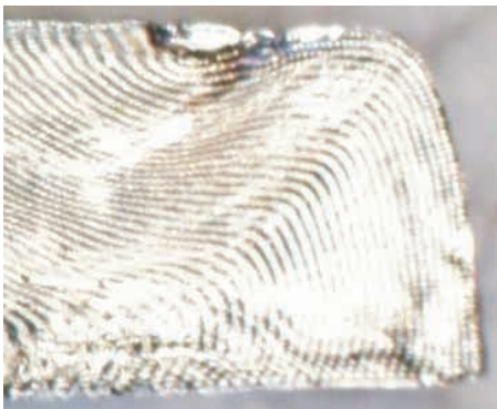
Fig. 8. Distortion of vertical bars, Copper single crystal ( \bar{\epsilon} = 0.90 )
