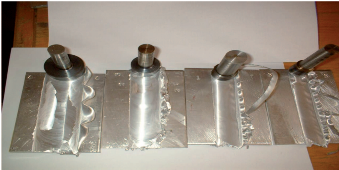
Fig. 5. Macroscopic pictures of the tested materials (Right to the left: 20 mm, 25 mm, 30 mm and 40 mm shoulder diameter)
