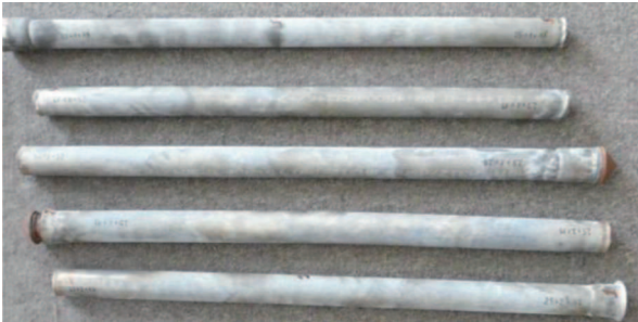
Fig. 3. Bimetallic bars after explosive welding
