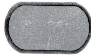
Fig. 13. View of a sample preformed oval strip designed for rolling 18 mm-diameter ribbed bars
