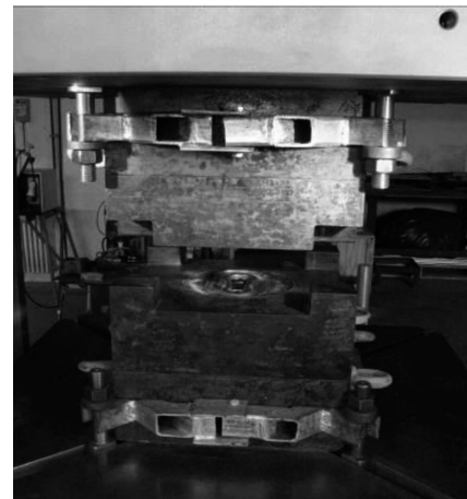
Fig. 2. A set of tools for die forging on a 2.5MN press – disassembled
