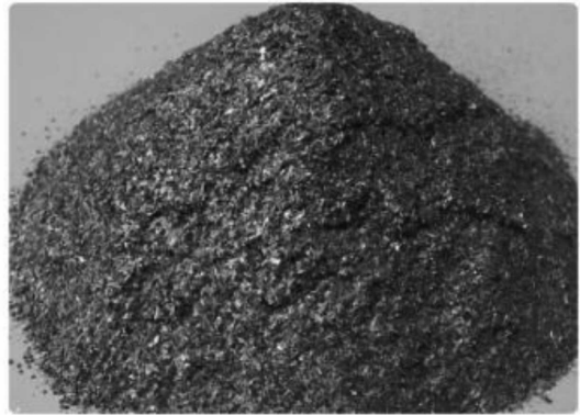
Fig. 3. Ribbon “chopped” into flakes in a cutting mill
