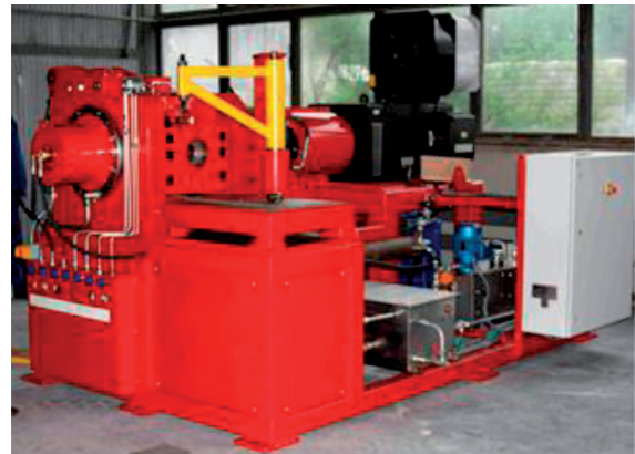
Fig. 4. View of the MC-260 device for continuous rotary extrusion made by Meltech-Confex Limited operating at IMN-OML
