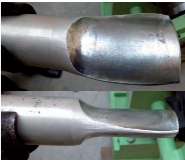
Fig. 10. Semi-finished product after rolling in oval impression for the first roll pass in the modified tools
