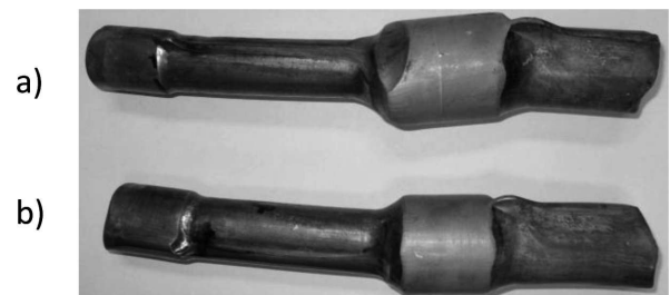
Fig. 13. Forgings from magnesium alloy AZ31 rolled in the forge rolling process: from billet with diameter 045 mm, b) from billet with diameter 042 mm
