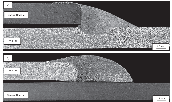
Fig. 4. Macrostructure of the overlap joints of Grade 2 titanium – aluminium alloy AW-5754 braze welded with AlSi12 filler metal \varnothing 2.4 mm, titanium on the top (a) titanium at the bottom (b), chemical etching using Kroll's reagent
