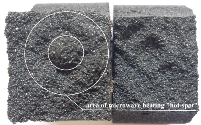
Fig. 4. Fracture surfaces of a dog-bone specimen (24 h) in the place of thermal destruction caused by microwave heating
