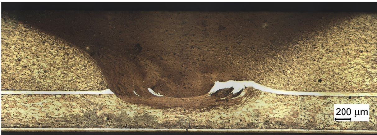
Fig. 3. Macrostructure of FSW aluminum joint
