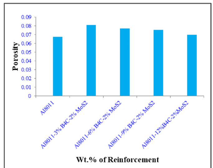
Fig. 9. Porosity in the Al8011- B_4C - MoS_2 composites
