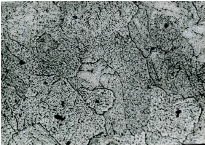
Fig. 13. Microstructure of continuous cast strip surface ( \times 100 )
