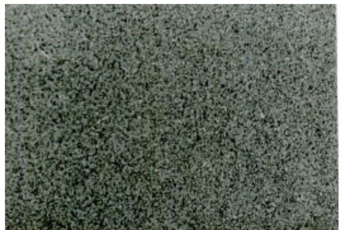
Fig. 11. Macrostructure of upper surface of continuous cast strip (×10)
