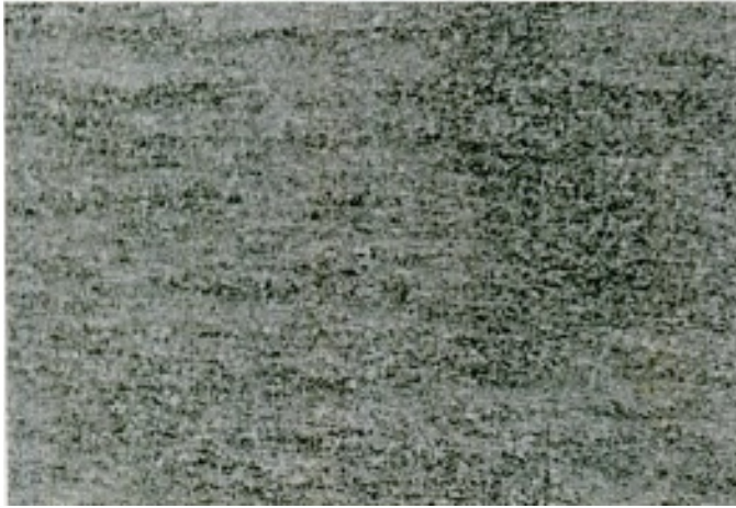
Fig. 12. Macrostructure of cold rolled non-annealed strip 2.5 mm ( \times 10 )
