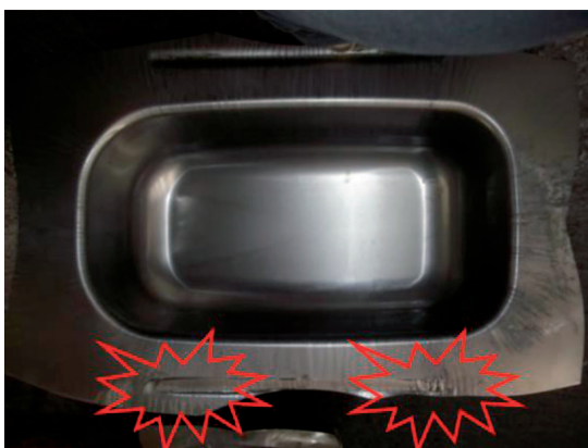
Fig. 15. Photo of final shape of a bathtub W1200 for the original die design with marked wrinkling area near geometrical drawbead
