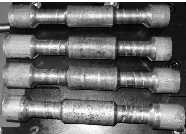
Fig. 8. Aluminum alloy 6061 stepped shafts produced by cross wedge rolling
