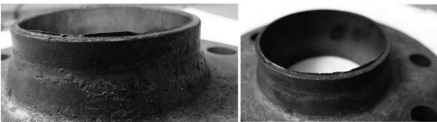
Fig. 13. Burr forming as result of bottom shearing
