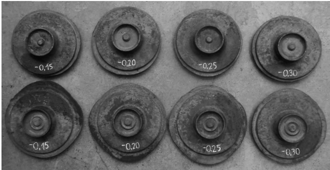
Fig. 12. Comparison of shape of upper part of flange with flash after second operation (top row) and third operation for every mass lowering (in kilograms)
