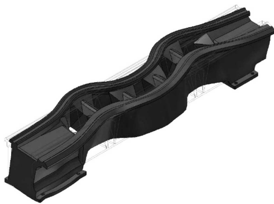
Fig. 13. F8 mode of the iron cast body – frequency 765 Hz
