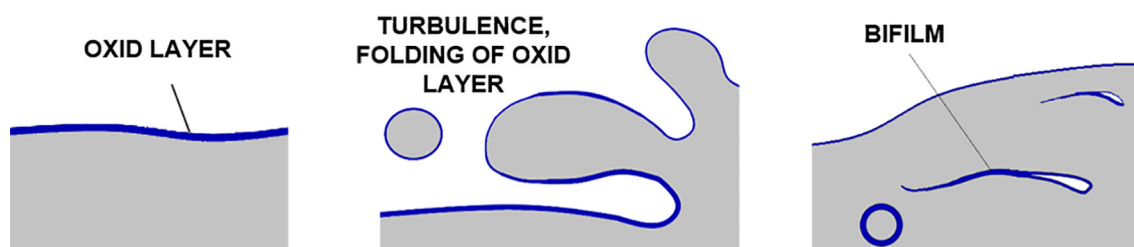
Fig. 1. Scheme of the bifilm origin
