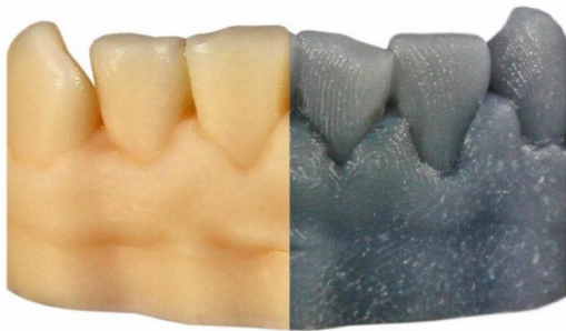
Fig. 5. Comparison of printing final result of DLP (left) and SLA (right) technique [13]
