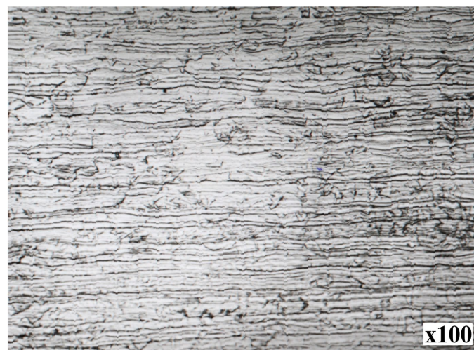
Fig. 5. The hot strip rolling (thermal treated); thickness: 0.85 mm
