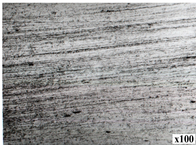
Fig. 4. The hot strip rolling; thickness: 0.85 mm
