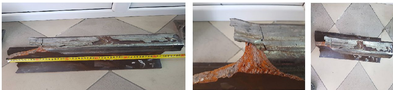
Fig. 2. Aspect of macroscopically analyzed areas and fracture surfaces
