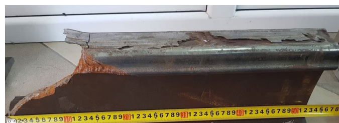
Fig. 1. Coupon aspect in the fracture zone
