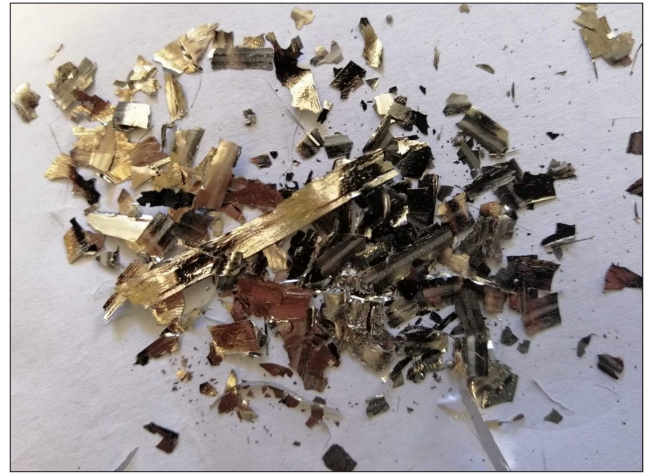
Fig. 2. The general aspect of the melt-spun \text{Fe}_{38.5}\text{Co}_{38.5}\text{Nb}_7\text{P}_{15}\text{Cu}_1 ribbons
