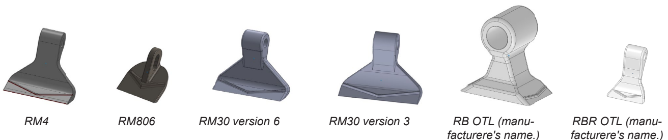
Fig. 2. CAD drawings of the developed constructions of hammerheads selected for the implementation
