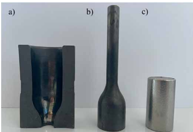
Fig. 1. View of: a) tool section, b) „pear”, c) charge material
