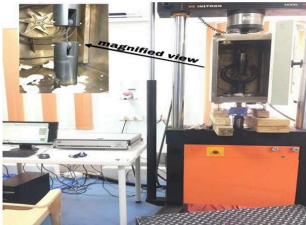
Fig. 2. Experimental setup for Computerized Universal Testing Machine and fractured samples at different temperature conditions
