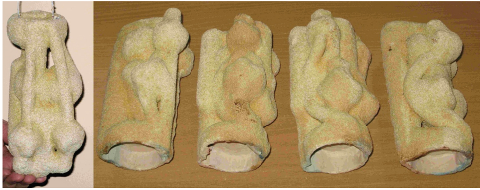
Fig. 30. Raw ceramic moulds before and after de-waxing
