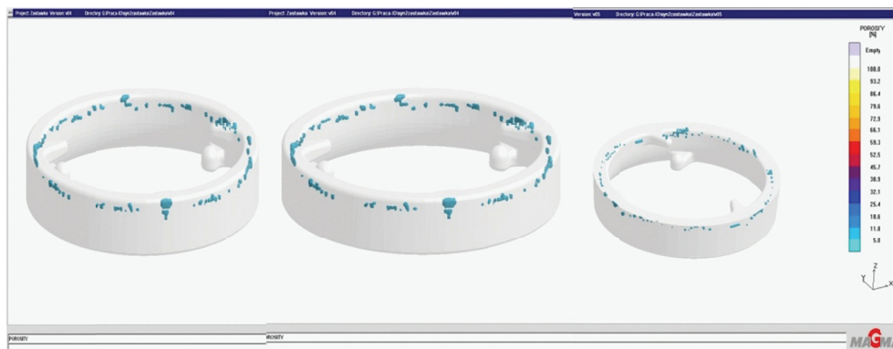
Fig. 10. The spatial distribution of shrinkage porosity occurring in casting and riser of different geometries on the example of a heart valve ring
