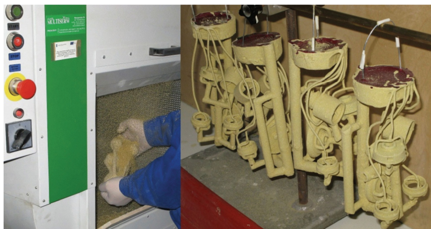
Fig. 29. Successive layers of the ceramic mould applied in a tumbling device (castings of the heart valve and hydraulic drive unit components)
