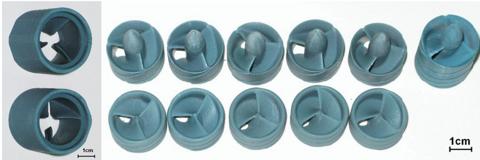
Fig. 6. Printed axial-flow pump elements: a stator and an impeller (after removal of the support material)
