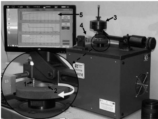
Fig. 4. Tribological tester working in a pin-on-disc configuration: 1 – specimen (pin); 2 – counter surface (disc); 3 – weights; 4 – tensometric force sensor; 5 – records of friction force
