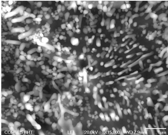
Fig. 6. Microstructure after schedule with heating rate 180°C/s and heating temperature 800°C – hardness 265 HV10. Large amount of fragmented pearlitic lamellae
