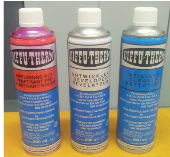
Fig. 7. Preparations set of the type „Diffu – Therm” used for penetrant testing of cracks
