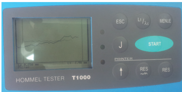
Fig.16. Visualization of the stereometric structure of the surface during the measurement
