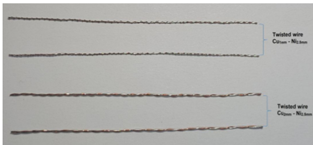
Fig. 1. The twisted wires of Cu and Ni wires were used in study
