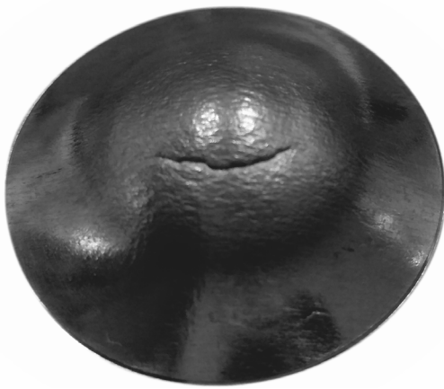
Fig. 7. Appearance of draw area after Erichsen test
