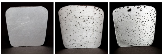
Fig. 4. Sample solidified in partial vacuum: Directly casted sample (left), 2x remelted (middle), 4x remelted (right)
