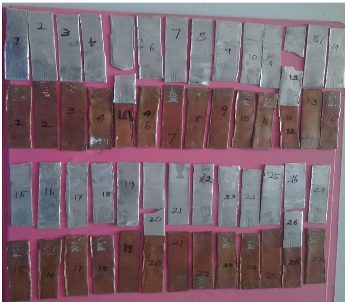
Fig. 5. Tensile strength tested specimen
