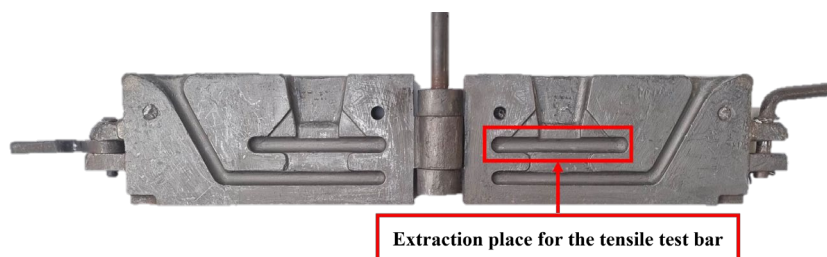
Fig. 1. Metal mold with extraction place for the tensile test bar
