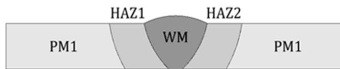
Fig. 1. Characteristic areas in the welded joint
