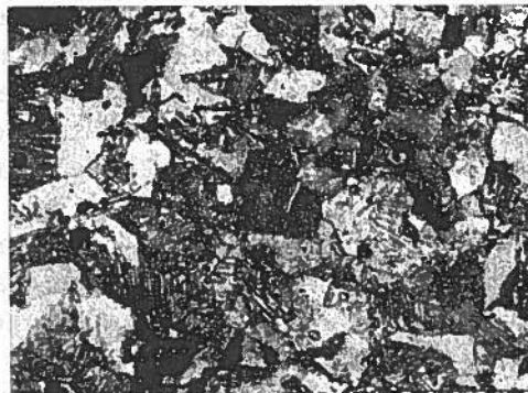
Fig. 8. Microphotographs of steel F; ferrite and pearlite (N 2 , 1000x)
