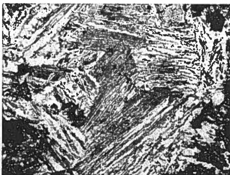
Fig. 9. Microphotographs of steel F; coarse pearlite ( N_2 , 1000x)
