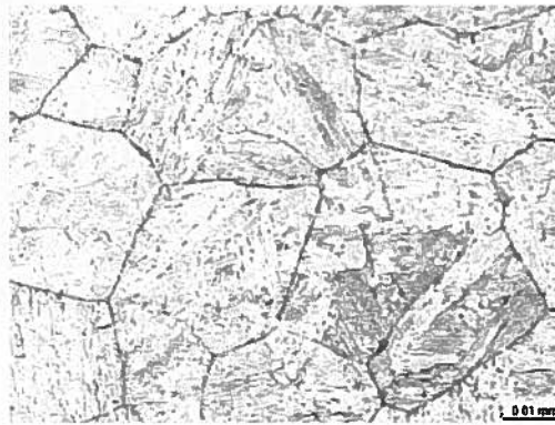
Fig. 5. Simulated HAZ area with coarse grained microstructure reheated to a temperature below A_{C1} (SRCGHAZ; T_{max2} < A_{C1} ). Martensite + carbides precipitated on grain boundaries (373 HV1)
