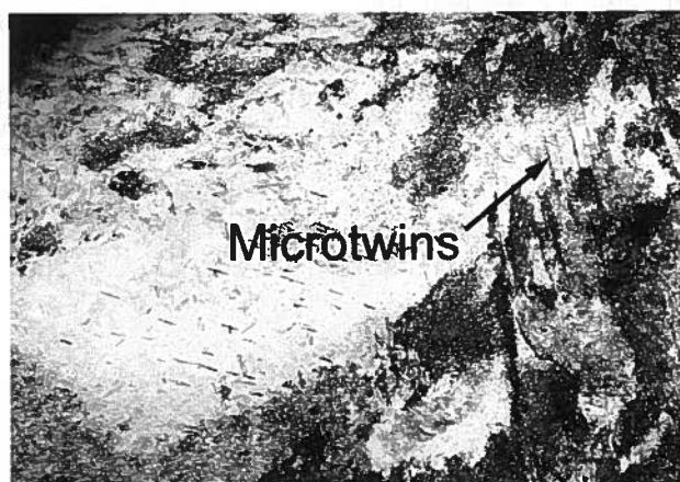
Fig. 16. SRCGHAZ area. Microtwins formed as a result of phase transformation of austenite to martensite
