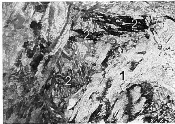
Fig. 12. Microstructure of P91 steel simulated by SRCGHAZ cycle: 1 – primary martensite, 2 – secondary martensite
