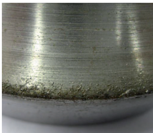
Fig. 1. Fragment of the surface of the forming roll with the glued Al-Si coating
