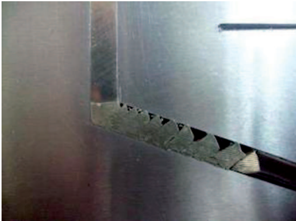
Fig. 6. Sample deformed by ECAP at temperature below 350°C
