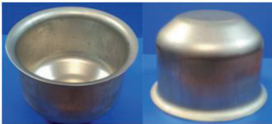
Fig. 14. The example view of bearing housing before trimming operation
