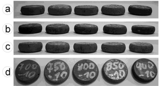
Fig. 5. Appearance of Cu-3Ti alloy specimens after compression at temperature in the range 700÷900°C up to a strain of 1.2 (70%) with strain rate of 0.1 (a), 1.0 (b) and 10.0 s -1 (c)
