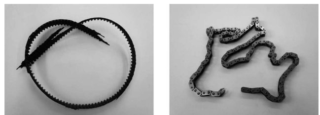
Fig. 4. Damage to belt and chain of timing system
