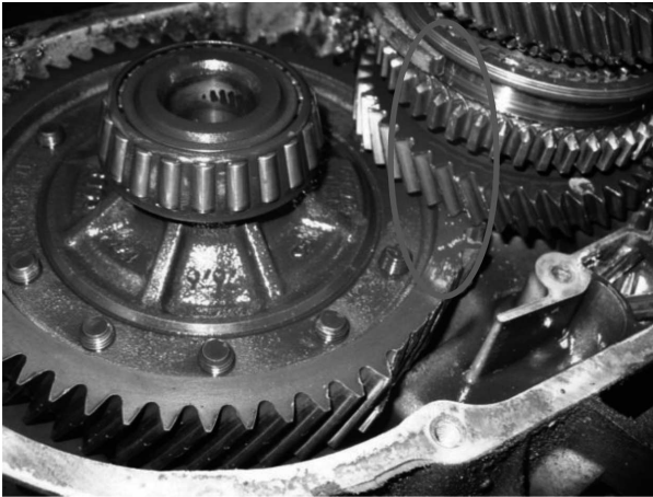
Fig. 14. Damaged bearing of main shaft
