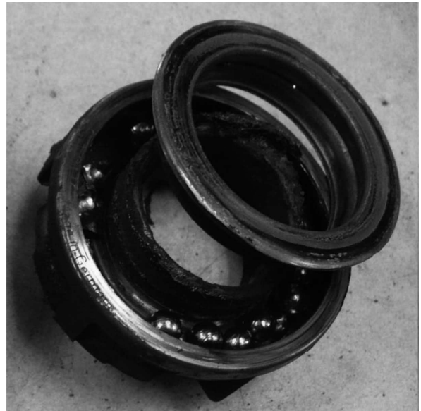
Fig. 7. Worn thrust bearing
