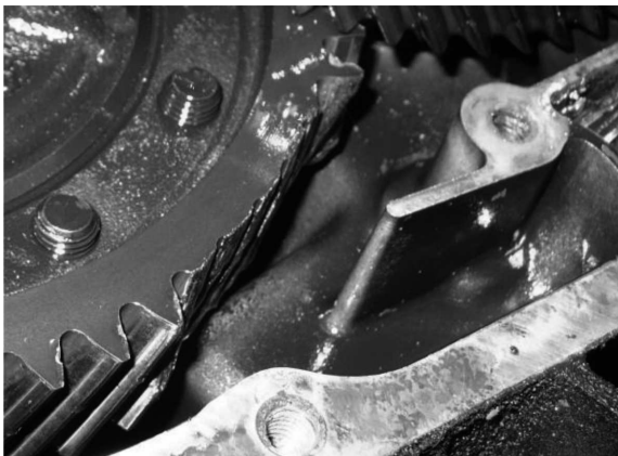
Fig. 15. Defected toothed wheels of main shaft
