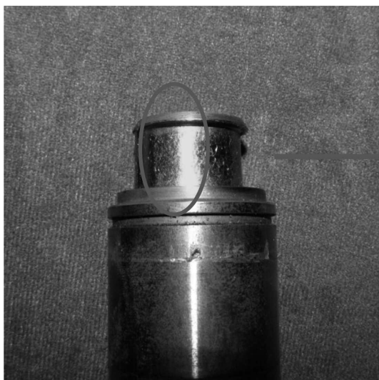
Fig. 12. Damage to main shaft bearing pin of gearbox
