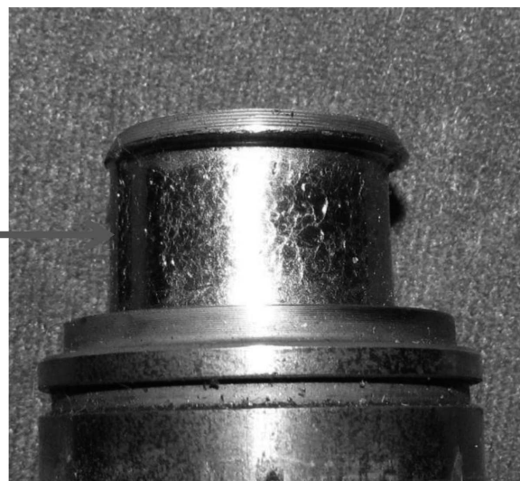
Fig. 13. Material wearing and change in diameter of pin
