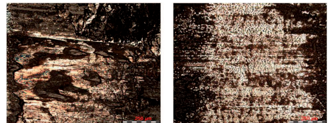
Fig. 9. Surface topographies of 12W (left) and 14W (right) samples after sliding distance of 500 m
