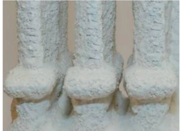
Fig. 7. Part of ceramic mould
