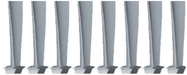
Fig. 6. *.CAD model of pattern assembly
