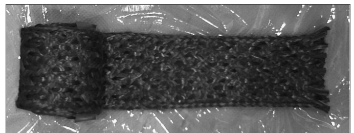
Fig. 5. Semi-finished product with bidirectional fibre arrangement obtained by means of plaiting
