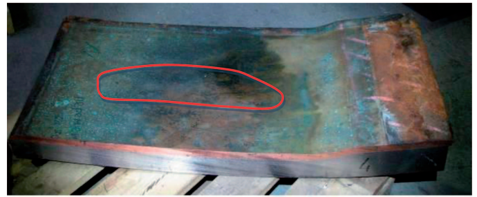
Fig. 11. The bimetallic blank cut along the central line with the zone of maximal wave formation
