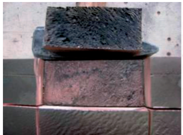
Fig. 9. Disclosed zone of rupture
