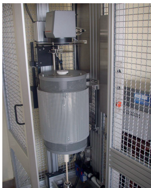
Fig. 3. Photograph of rotational viscometer used in investigations
