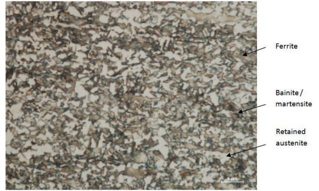
Fig. 3. Structure of wire of steel with a carbon content of 0.43% after two-stage heat treatment
