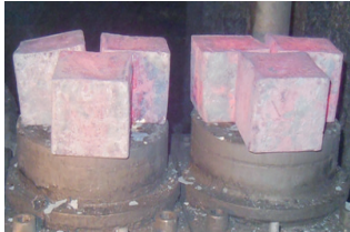
Fig. 11. Heating the tools by heated preforms
