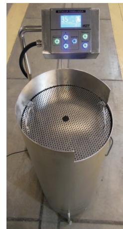
Fig. 20. A cooling-lubricating device regulating the supply of the lubricant agent
