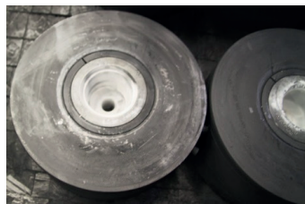
Fig. 14. Tools coated with foam used in welding without the necessity of pre-heating
