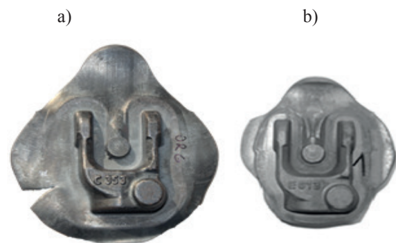
Fig. 10. Comparison of the forging shape: a) before tool modification and b) after tool modification [8]
